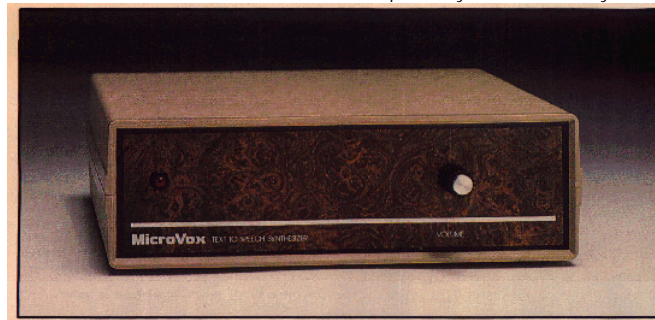
Photo 1: An assembled Microvox speech synthesizer, which can pronounce lists consisting of English words from their representation as ASCII characters according to fixed pronunciation rules. The Microvox contains a general-purpose 6502-based microcomputer programmed to control the Votrax-SC-01A-based speech-synthesis circuitry.
