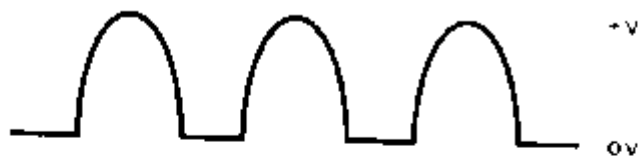
Figure 8: Voiced Sounds from the Glottis. Sounds which have definite pitch are called voiced sounds. In the natural larynx, these sounds are generated by the vocal chords and drive the vocal tract at the glottis. In an electronic analog, the voiced sounds can be generated by a programmable counter (to set the frequency) which in turn creates a sine wave of the same frequency. A rectified sine wave is a good source for the glottal pulses used in the electronic model of a larynx used in the author's approach to speech generation.
